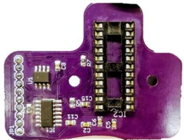
b. Completed TCD1304 Interface Circuit Figure 5. Designed and Fabricated Circuit
