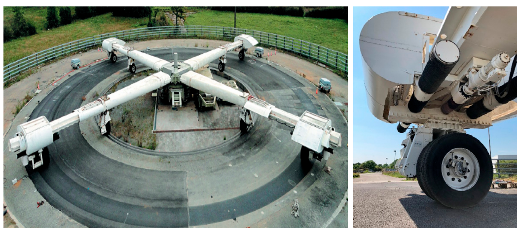
Figure 2. Fatigue carousel for accelerated pavement tests, Nantes—France.
