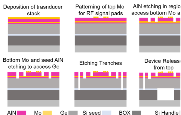
Figure 4: Fabrication process flow of for implementation of AlN-on-Ge delay lines. Top Mo SPUDTs serve as RF signal pads and bottom Mo serve as GND pad. The DC bias is applied by accessing Ge. The DC and RF fields are isolated through a 20nm AlN layer.
