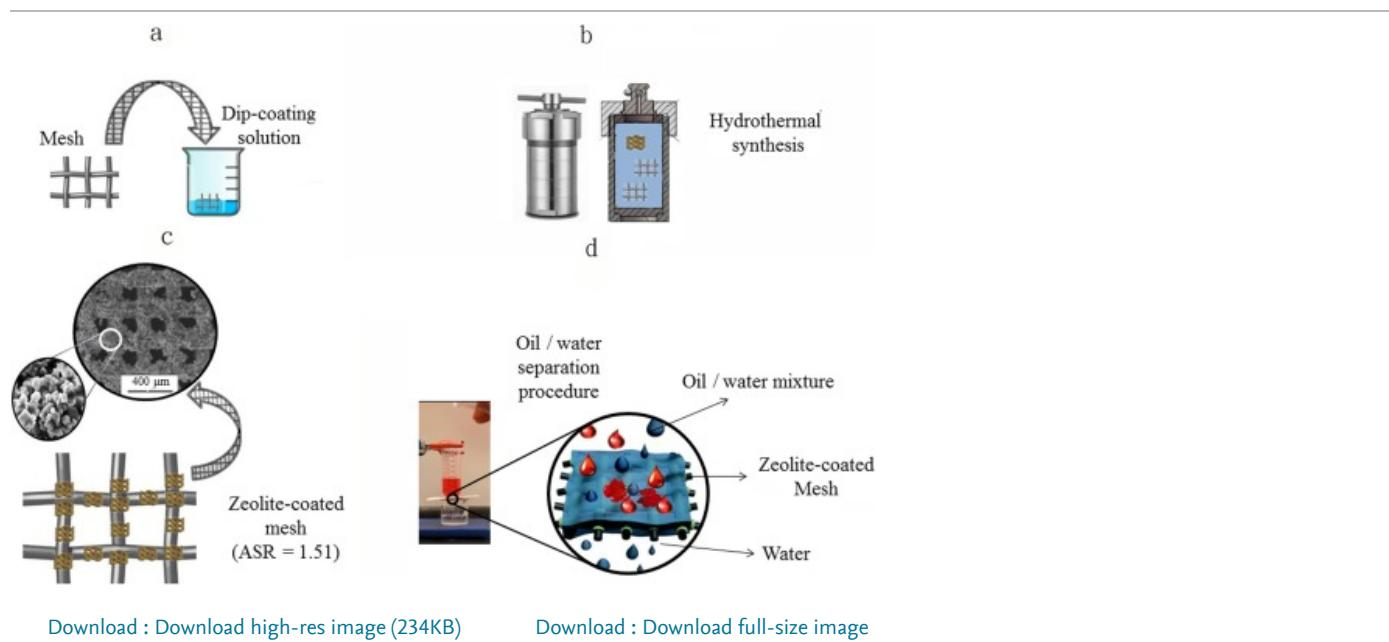
Fig. 1. Schematic illustration of the synthetization of the NaA zeolite coated mesh (a) dip-coating, (b) hydrothermal synthesis, (c) zeolite-coated mesh, and (d) oil/water separation procedure.
