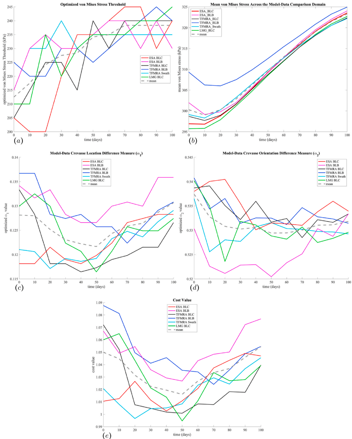
Fig. 10. Evolution of model and optimization values over each 100 day model simulation. ESA-Baseline-C (Red), ESA-Baseline-B (magenta), TFMRA-Baseline-C (black), TFMRA-Baseline-B (blue), TFMRA-Swath (cyan) and LMG-Baseline-C (green). The gray dashed line plots the mean value across all model experiments at each time. (a) The optimized von Mises stress threshold ( \sigma_{threshold} ). (b) Mean von Mises stress measure ( \bar{\sigma}_{vm} ) across the model-data analysis domain. (c) The model-data crevasse location difference measure ( \alpha_1 ). (d) The model-data crevasse orientation difference measure ( \alpha_2 ). (e) The minimized cost value associated with each time. (For interpretation of the references to color in this figure legend, the reader is referred to the Web version of this article.)
