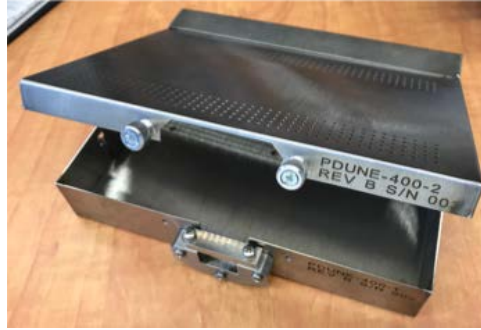
Figure 4.25. Prototype CE box used in ProtoDUNE-SP
