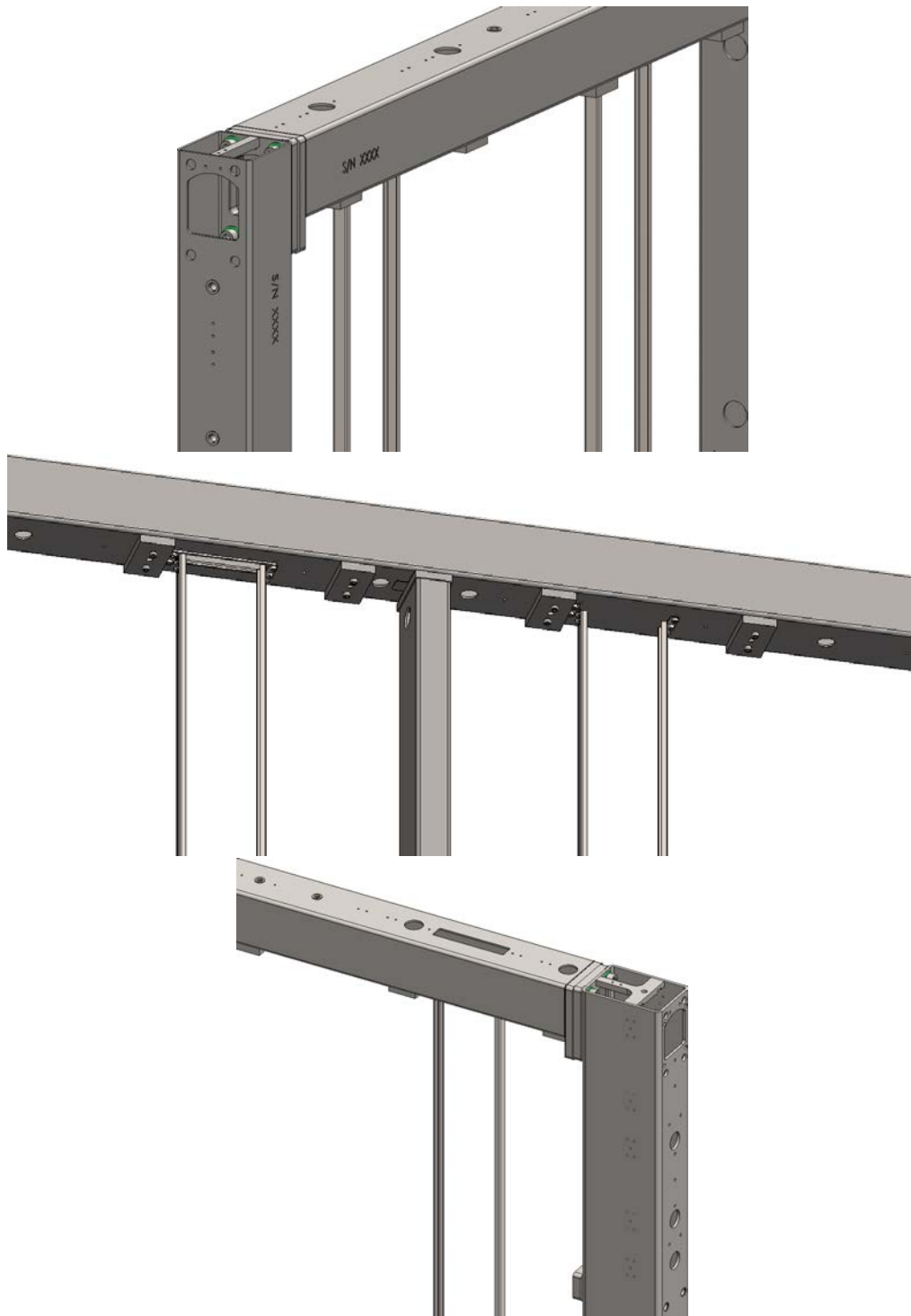
Figure 2.8. APA frame construction details. Top: the corner joint between the foot tube and the side tube. Middle: the joint between the side tube and a rib. Bottom: the joint between the head tube and the side tube.
