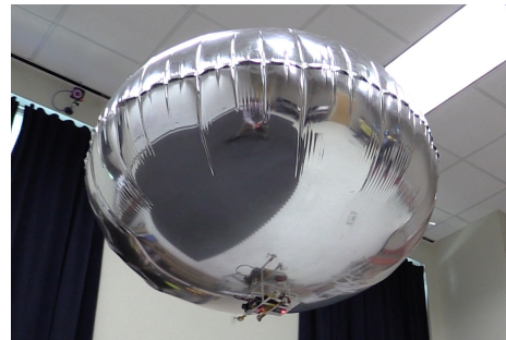
Fig. 1: The Georgia Tech Miniature Autonomous Blimp (GT-MAB). The GT-MAB consists of two major components, the envelope and the gondola. The envelope is the upper balloon-like portion that is filled with helium so that the platform can fly for long durations. The gondola houses the sensors, motors, microcontroller, camera and communication modules.
