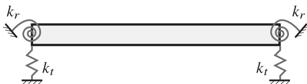
Fig. 2 Schematic of a beam with flexible boundary conditions
