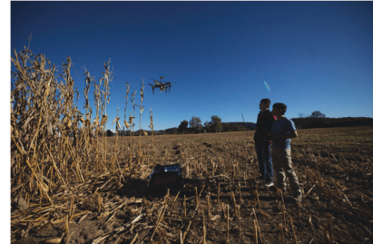
Fig. 1. Single quadcopter can fly over a farm and measure the height of the crop using a LIDAR sensor.
