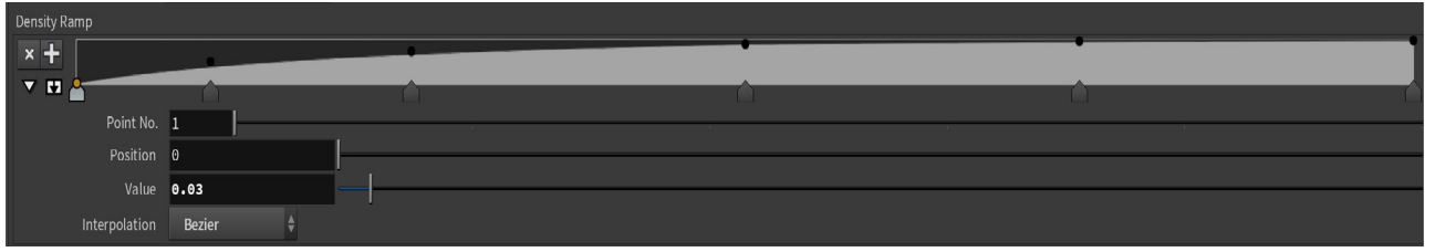
Fig. 8. The density ramp, mapped to opacity in the shader, where density values increase from left to right from 0 to 3.4—its max value after pre-processing. The higher the ‘Value’ indicated by the ramp, the more opaque (less transparent) each particle at that particular density will be. Values are determined by a cubic Bezier curve with the control points P_0 = (0, 0) , P_1 = (0, 0.2) , P_2 = (0, 1) , and P_3 = (1, 1) . The ‘Interpolation’ between each point is also set to ‘Bezier’. Less dense particles (typically near the outer edges of the synestia) are less opaque, and more dense particles (typically concentrated in the center of the synestia) are more opaque.
