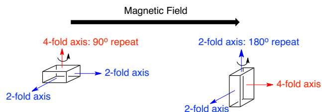
Figure 6. Rotational symmetry of crystal sample placed in the EPR cavity.
