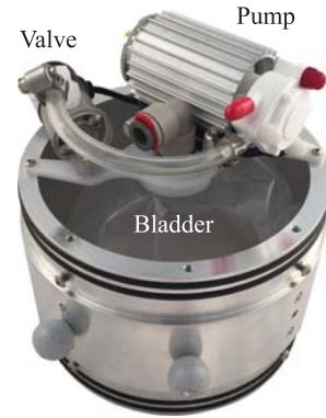
Fig. 3: CephaloBot buoyancy ring shown with pump, valve, and bladder. Pressure sensors (not shown) used to monitor bladder pressure and pump flow rate are installed in-line between the pump outlet and the bladder inlet.
