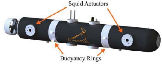
Fig. 2: Render of the CephaloBot AUV with new buoyancy engine ring modules. Each ring houses a buoyancy bladder, valve, and pump. Like the squid actuators on the vehicle, the buoyancy engine incorporates compliant components in its design.
