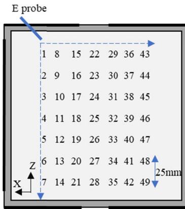
Fig. 4. Experimental validation of the E-field distribution using an E-field probe at different locations of the generator.
