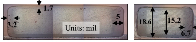
Fig. 4. Cross section of the divided 0603 capacitor under a microscope with 5× magnification [20].
