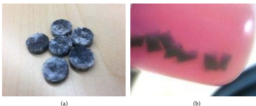
Figure 2. (a) Pellets with \text{KMnO}_4 encapsulated in PCL; (b) Pellets release \text{KMnO}_4 in water.
