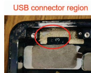
Fig. 18. Electric connection between USB board and chassis.
