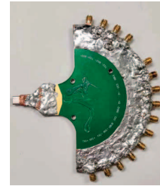
Fig. 8. (a) Measurement setup for passive noise transfer function. (b) Shielded Type-C plug to SMA fan-out board.
