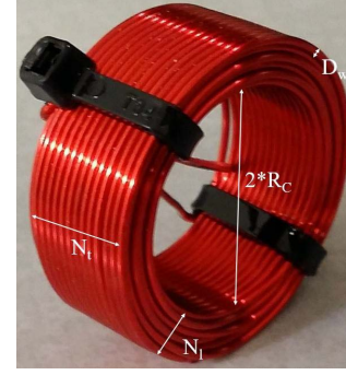
Fig. 5. Photograph of a typical coil illustrating the parameter definition of the coil model.
