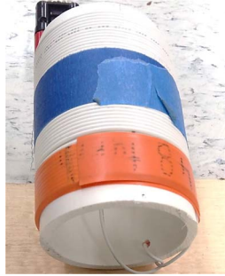
Fig. 3. Magnetic field detection coil.
