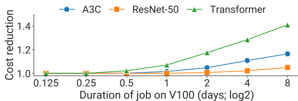
Figure 6: Average cost reduction from allowing dynamic switching of instance type, cloud, and availability zone during training, while varying job duration. Longer jobs are able to make use of greater variability in prices over longer horizons, consequently leading to larger cost reductions. The right two bars in Figure 5 shows the impact of dynamic switching for jobs with a duration of 4 V100-days.
