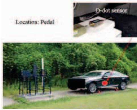
(b) IEMI measurement setup
