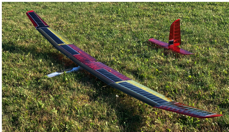
Figure 21. The UIUC-TUM Solar Flyer aircraft shown with solar arrays.
