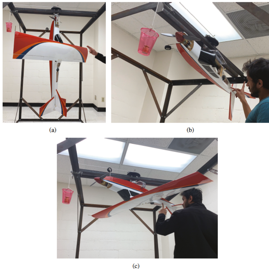
Figure 12. Moment of inertia testing of the flight-ready, instrumented Great Planes Avistar Elite about the (a) roll axis, (b) pitch axis, and (c) yaw axis.
