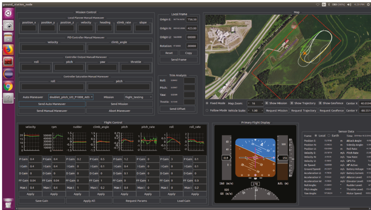
Figure 13. Screenshot of ground station interface with aircraft setup up for up-down 1000 ms, 50% elevator deflection doublet maneuver.
