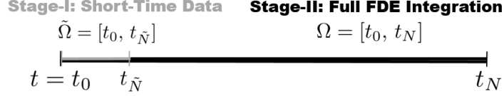
Figure 1.: In Stage-I, the scheme captures the singularities for the short time-domain \tilde{\Omega} , given the short initial data. In Stage-II, the framework uses the singularities obtained in Stage-I for full time-integration of the FDE over \Omega .
