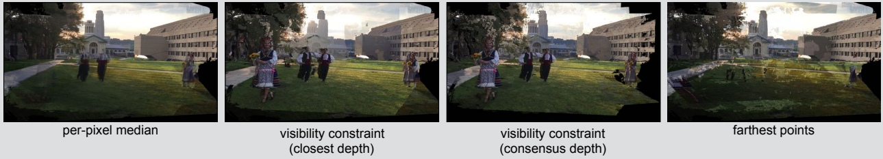
Figure 4. Instantaneous Foreground Estimation: Given multiple stereo pairs and a target camera view, there are three steps for estimating instantaneous foreground. (1) We estimate disparity for a rectified stereo pair using an off-the-shelf disparity estimation approach [50] and project it to a target camera view using standard 3D geometry [19]. (2) We repeat Step-1 for the \binom{N}{2} stereo pairs. (3) A crucial aspect is to fuse the information from multiple projections to generate a comprehensive instantaneous foreground. A simple per-pixel median over the multiple projections leads to a loss of dynamic information because of the poor 3D estimates (shown in first column). We propose a visibility constraint using painter’s algorithm. The visibility constraint builds a per-pixel cost volume of depth. It is natural to have multiple depth values for a given 2D pixel location in the image. For each pixel location, we consider the 3D point corresponding to the closest depth to the target camera view. Due to noisy 3D estimates, it often leads to ghosting artifacts (shown in second column). However, we have multiple views and we ensure consistency in the depth values of the closest 3D point for projection to a 2D pixel location by analyzing their visibility. As shown in third column, this consensus in depth leads to improved results. Finally, we also show the projection of pixels corresponding to the farthest points (fourth column) for a given pixel location to illustrate cost volume of depth. Note that it removes dynamic information in the scene.
