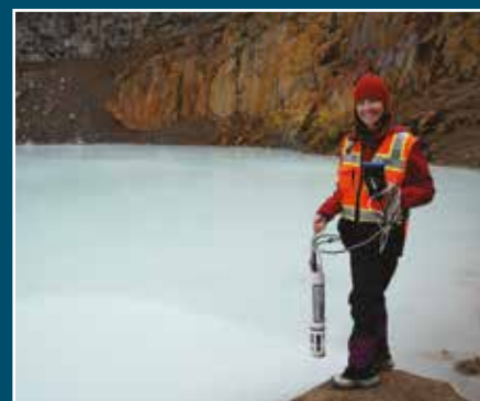
Dr Duhamel uses a multiparameter water quality sonde to measure environmental conditions within an acidic volcanic lake.
