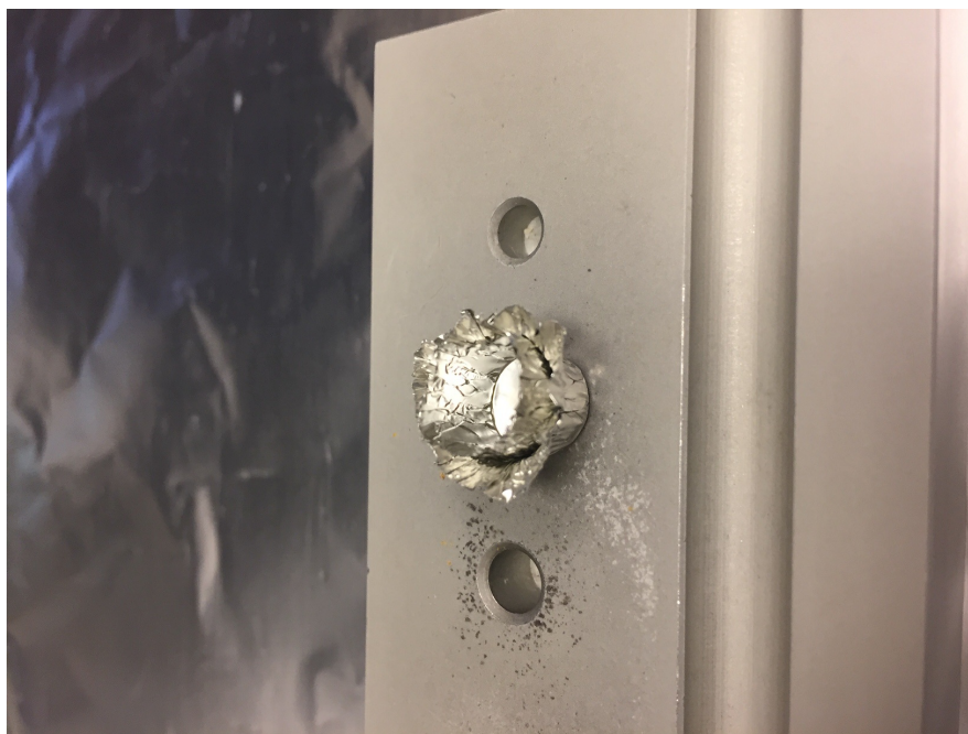
Figure 6 An example of a tin capsule doublet, where one 9 mm x 10 mm tin capsule is placed within another to avoid the liquid host fraction from leaking out during the drying process.
