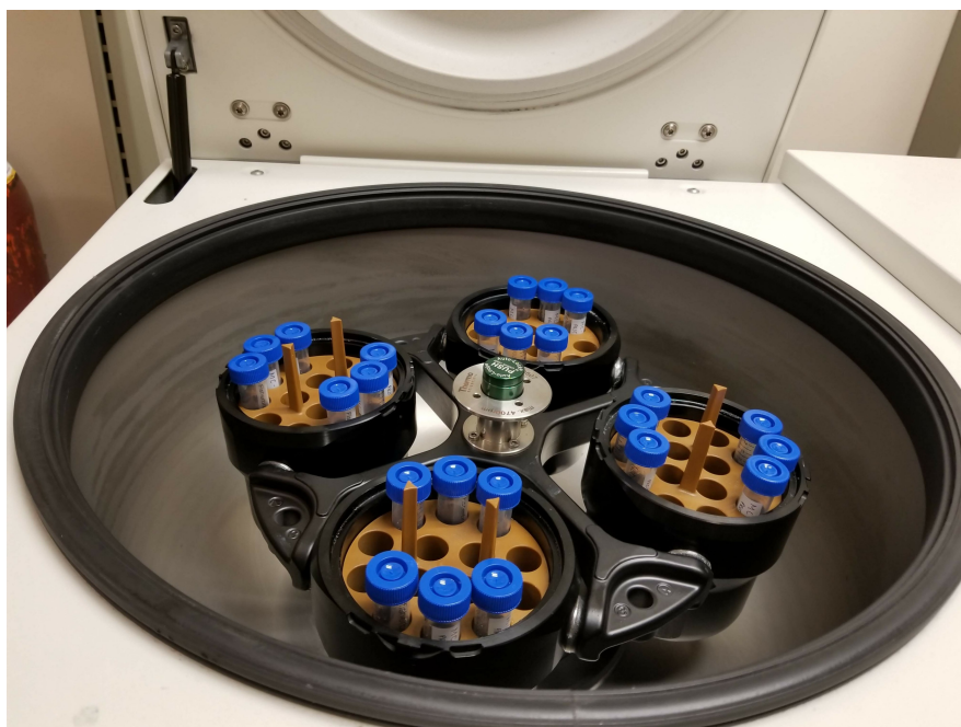
Fig. 4. Example of balanced configuration of 15 ml centrifuge tubes inside a refrigerated swing-bucket centrifuge.
