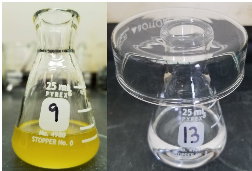
Fig. 14. Left: E-Flask with organic phase from coral sample drained from the separatory funnel. Right: Example of how Petri dish can be used as a lid on each of the E-Flasks . Note, E-Flask #13 is the control, hence why the liquid has a clear color in this example.
