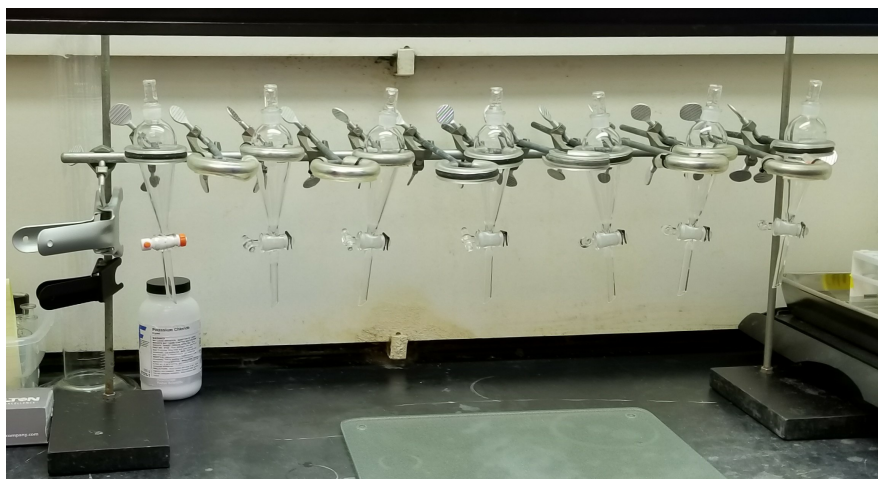
Fig. 8. Retort stand assembly for holding 13 separatory funnels within fume hood. Only 7 separatory funnels are shown above, each with a glass stopper and a Teflon or glass stopcock.
