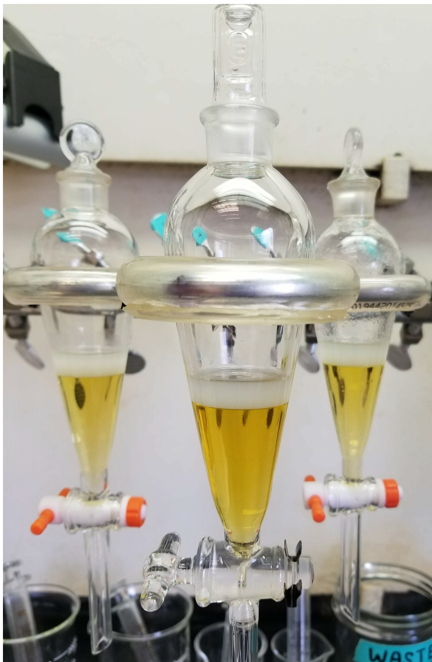
Fig. 13. White aqueous phase sits above the yellow organic phase of the solvent mixture in the separatory funnel.
