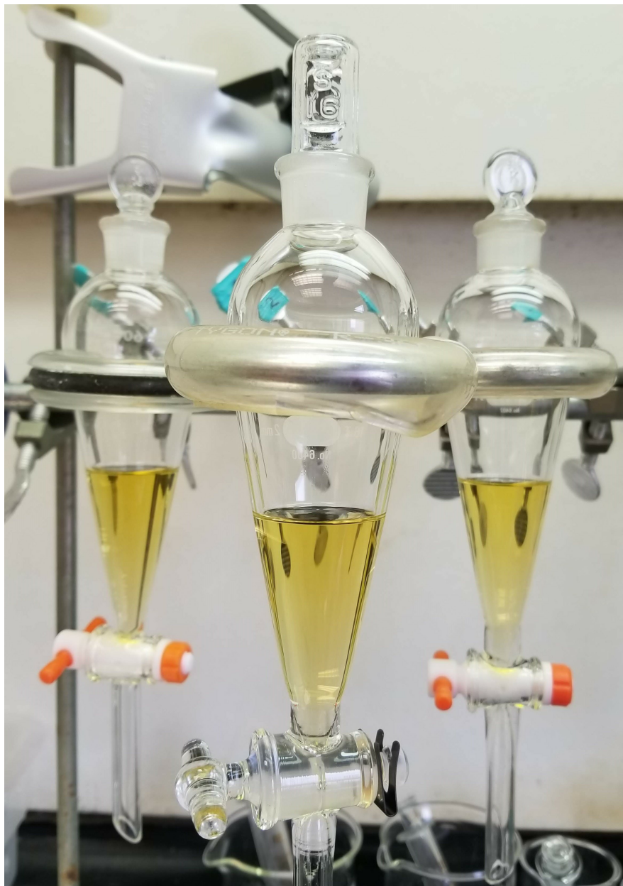
Fig. 12. Separatory funnel with filtered lipid extract inside, stopcocks in the closed position, and stoppers in place.
