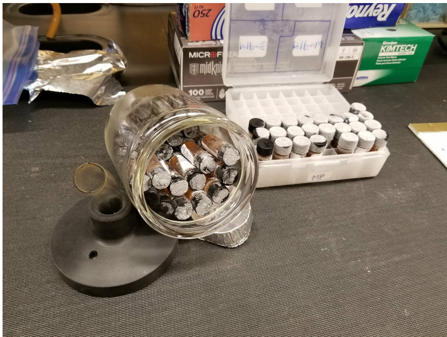
Fig 2. By tilting the wide-mouth flask on its side, it is easier to assemble the Freeze-Drying Vials inside in two layers.
