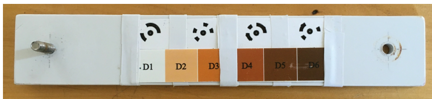
Single Tomahawk face with 4 Metashape markers and 1 side of a CoralWatch Coral Health Chart. White electrical tape holds down targets and color card while ensuring all markers and colored sections are visible.
