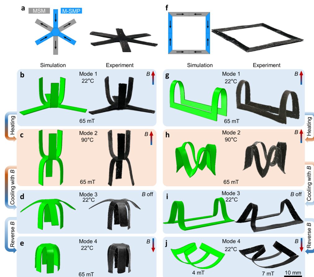
Figure 3. Schematic designs, simulations, and experiments of M-SMP/MSM composites for multimodal pop-up actuation. (a–e) Asterisk design with alternating material distribution and magnetization directions. (f–j) Square frame design with inward-pointing magnetization directions.
