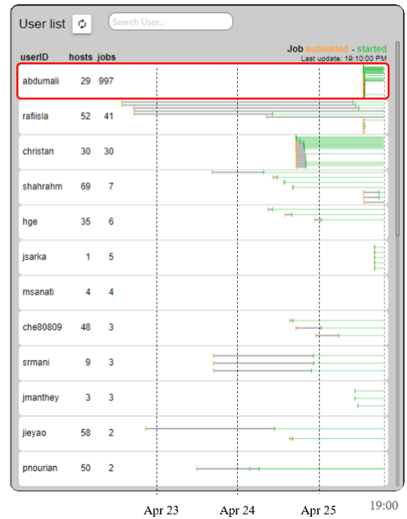
Fig. 2. Time series visualization for HPC job scheduling data: Gray horizontal bars represent waiting periods while green bars are currently active jobs.
