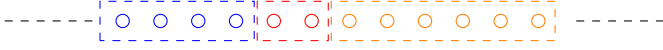
Fig. 6. OSA illustration: points are ordered w.r.t. LLR values. Each color represents a cluster and LLR value difference in each cluster is less than l_s .
