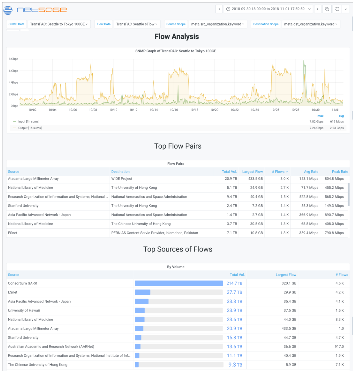
Figure 7: Partial Flow Analysis [46] Dashboard showing SNMP and flow data that identifies recurring data transfers that were part of a VLBI astronomy research project between Italy and Japan over the TransPAC4 link between Seattle and Tokyo in October 2018.
