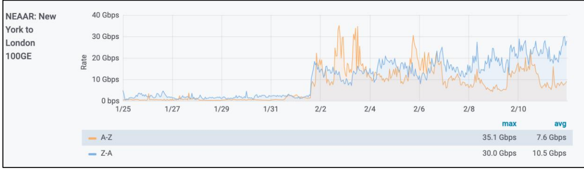
Figure 5: Traffic volume graph using SNMP data to show the increase in network traffic on the NEAAR link between New York and London for January-February 2018 [44]. Note the two colors indicate traffic in different directions on the circuit.
