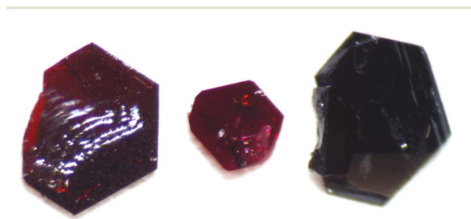
Fig. 1 Optical micrograph of \text{K}_2\text{Mn}_3(\text{VO}_4)_2\text{CO}_3 , \text{Rb}_2\text{Mn}_3(\text{VO}_4)_2\text{CO}_3 ( I ), and \text{K}_2\text{Co}_3(\text{VO}_4)_2\text{CO}_3 ( II ). For scale, the center crystal is about 1 mm across in width.
