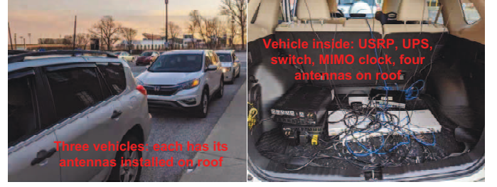
Fig. 10: A vehicular testbed consisting of three vehicles.
