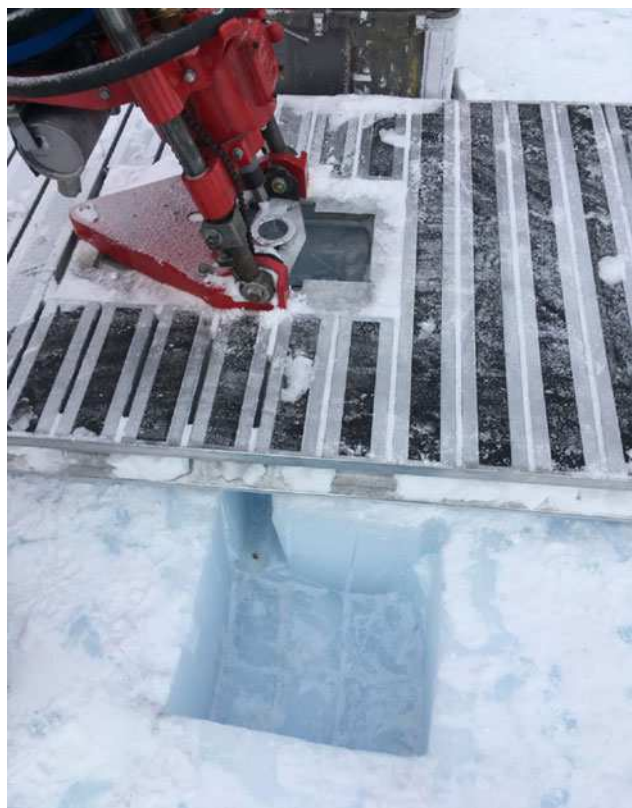
Fig. 6. An ice sump was cut into the surface of the blue ice to collect the fluid and chips as they were pumped to the surface.
