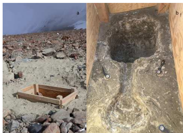
Fig. 7. (a) At the Ong Valley drill sites a layer of sediment was covering the ice surface. Once the ice was exposed, a timber barrier was built to support the drill rig and prevent loose sediment from falling into the borehole. (b) A channel was carved into the marbled ice to direct the drill fluid to a sump where it could be pumped into the filter tank. The borehole was drilled into the center of the bowl at the bottom of the image.
