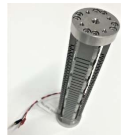
(a) Simplified phase diagram of CO 2 (b) Piezoelectric actuator
