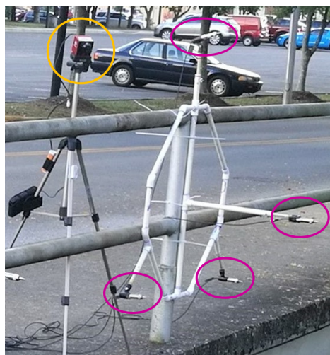
Figure 2. Thermal camera (in yellow circle) and one array of microphones (in magenta ovals).
