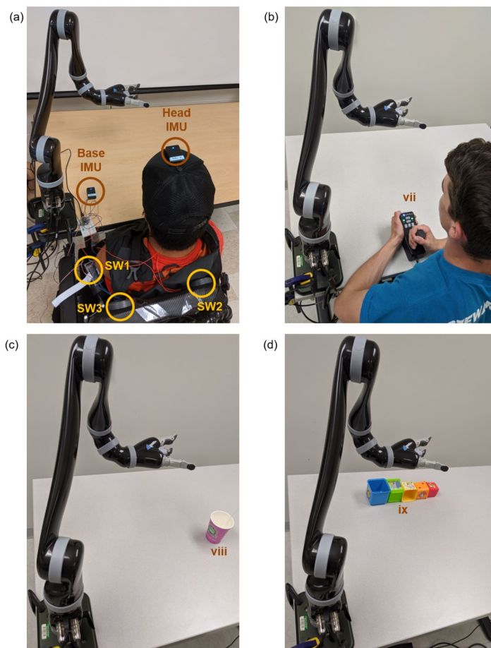
Fig 1. Interfaces for controlling the robot and experimental setup for the drinking and stacking tasks. (a) Interface for main participant using the head-joystick. A head mounted IMU was used to control the robotic arm, and switches (SW1, SW2, SW3) placed behind the shoulder were used to toggle between different control modes and for control of the grasper. (b) Interface for control participant using the manual joystick. (c) Initial layout of drinking task. Participants had to use the robotic arm to grasp the cup and bring it to the mouth. (d) Initial layout of stacking task. Participants had to use the robotic arm to stack the five blocks on top of each other in order of decreasing size with the biggest block at the base.
