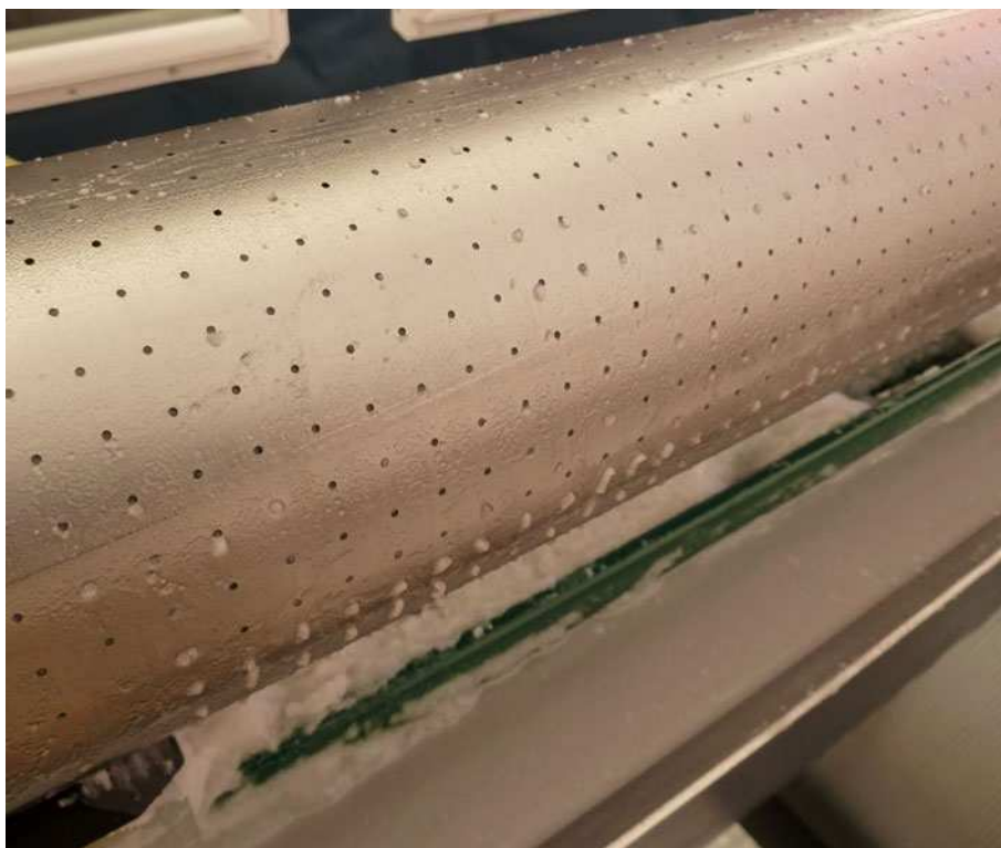
Fig. 13. Vented chips chamber tube with fine cuttings seeping from the vent holes.
