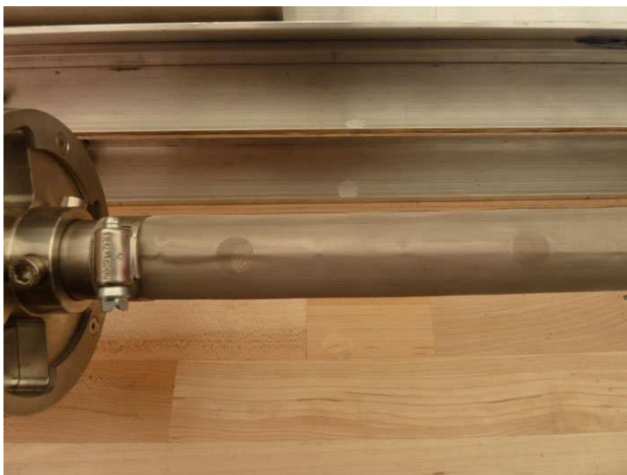
Fig. 14. Close-up view of the hollow shaft with 12 mm diameter vent holes covered by an 80-mesh filter screen.
