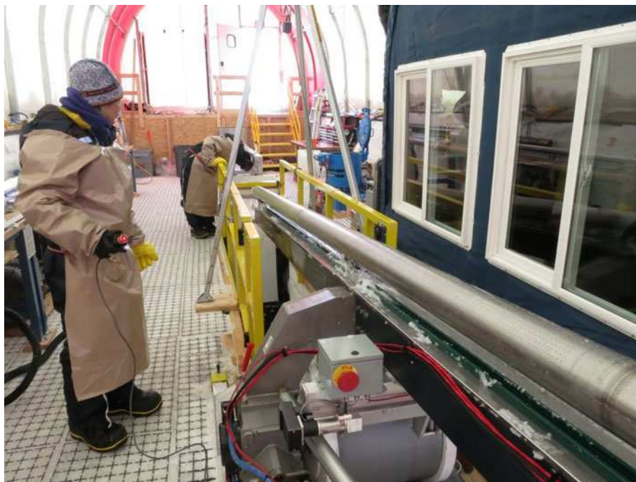
Fig. 5. The driller in the foreground begins to tilt the tower as the other driller does one final inspection of the cutter head.
