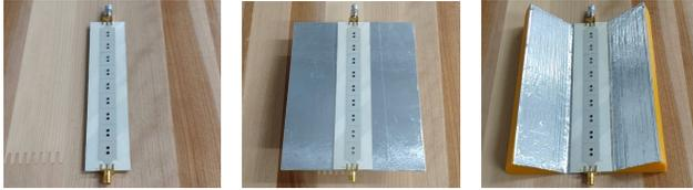
(a) Without ground (b) Extensions at 0° (c) Extensions at 40° plane
