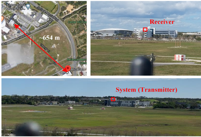
Fig. 7. Communications tests setup: rooftop of two buildings from Embry-Riddle Aeronautical University at approximately 650 meter of distance.
