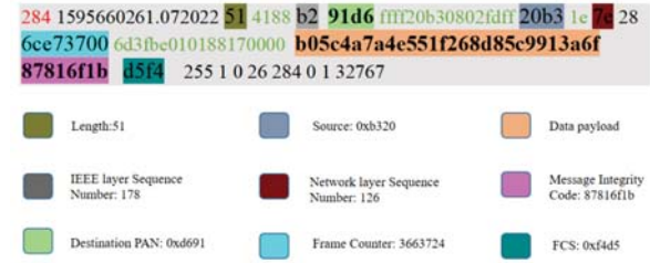
Fig. 11: Characteristics of captured frame for turning OFF the Philips Hue bulb.
