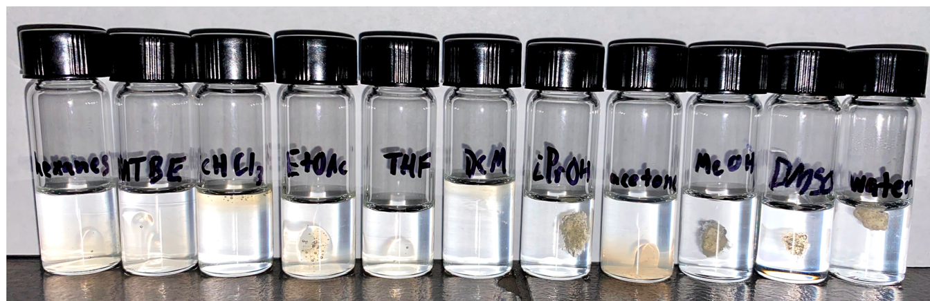
Figure 5. Swelling tests of 20–30 mg of cross-linked poly(myrcobdi) after ~60 min in a variety of solvents lined up from left to right with ascending dielectric constants.
