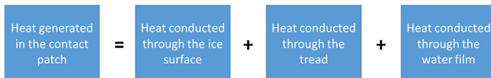
Fig. 3. Thermal balance equation at the contact patch based on the principle of heat balance (Bhoopalam et al., 2016).
