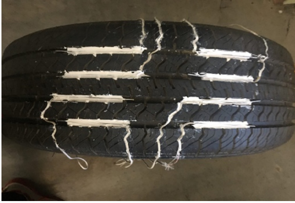
Fig. 4. Eight thermocouples installed to monitor the temperature changes at tread.
