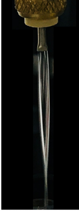
Fig. 10 Photo of a 120 \mu\text{m} thick water film formed by a water jet with a flat nozzle [62]. The laser beam is focused into the center of the film where is flat and stable
