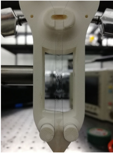
Fig. 2 Photo of the water film. Two aluminum wires are separated by 4\ \text{mm} . The thickness of the water film is controlled by the water flow rate
