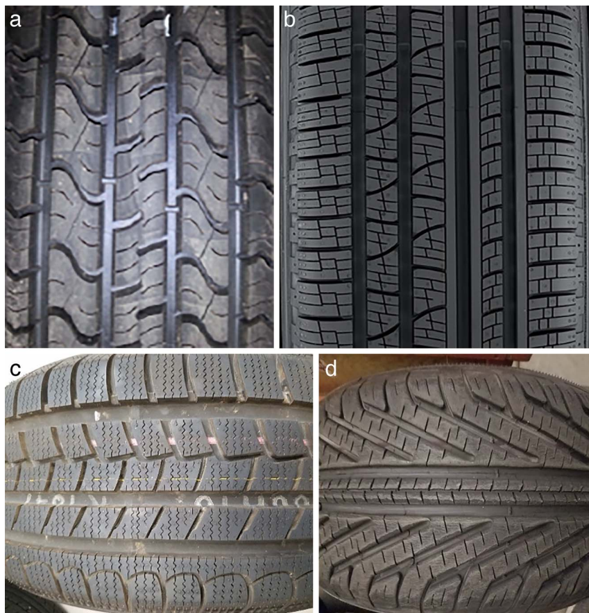
FIG. 2 — Tread design of candidate tires used for the study.
