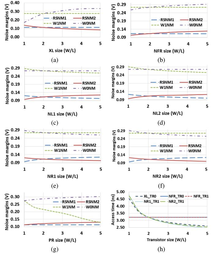
Figure 5: Noise margins of the SRAM cell versus the sizes of (a) XL (b) NFR (c) NL1 (d) NL2 (e) NR1 (f) NR2 (g) PR. (h) Access time of the SRAM cell versus the transistor sizes.
