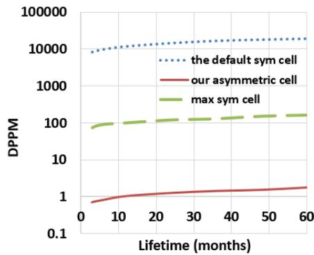
Figure 10: DPPM comparison for 2MB SRAM arrays when value “0” is stored in all cells for 75% of the time.
