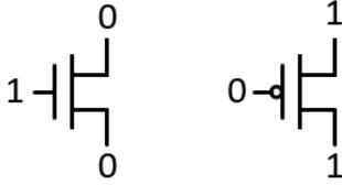
Figure 1: Stress state for NMOS transistor and PMOS transistor.
