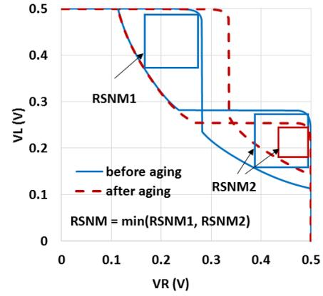
Figure 3: The butterfly curve of a 10T ST SRAM cell indicating RSNM before and after aging.
