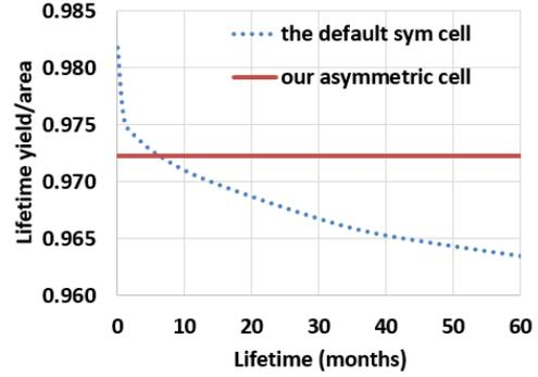
Figure 9: Lifetime yield per area comparison for 2MB SRAM arrays when value “0” is stored in all cells for 75% of the time.
