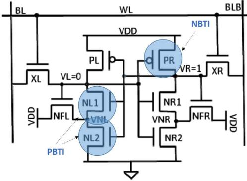
Figure 2: 10T ST SRAM cell.
