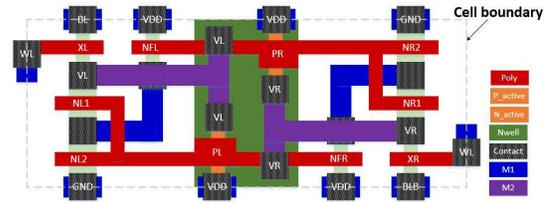
Figure 8: Layout of 10T ST SRAM cell.
