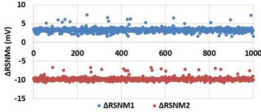
Figure 7: The read noise margin changes after 60 months usage for 1000 monte carlo SRAM cell instances with process variations.
