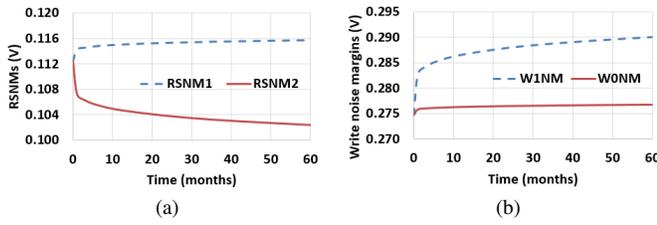
Figure 4: (a) Read noise margins, and (b) write noise margins through lifetime for a symmetric 10T ST SRAM cell when value “0” is stored in the cell for 75% of the time.
