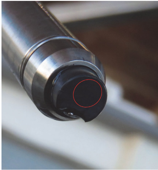
Fig. 2 Close-up look at the tip of the robust and fast-responding dual O 2 -temperature sensor developed for aquatic eddy covariance measurements. A replaceable black plastic disc contains the O 2 sensing foil, which is marked with a red circle and has a diameter of 5.0 mm. The < 1 mm shiny thermistor tip is seen below it (credits: photo by the authors).
