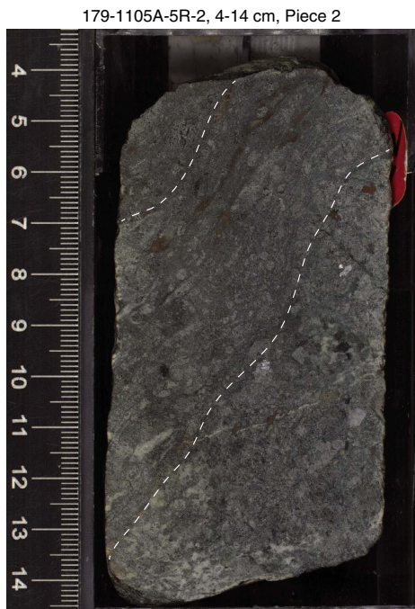
Figure F34. High-temperature solid-state foliation defined by the orientation of plagioclase layers and sigmoidal clinopyroxene grains, immersed in a fine-grained plagioclase + clinopyroxene + olivine + oxide mixture, Hole 1105A. Note sharp contact of shear zone with less crystal-plastically deformed gabbro at bottom of image.
