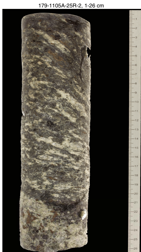
Figure F34. High-temperature solid-state foliation defined by the orientation of plagioclase layers and sigmoidal clinopyroxene grains, immersed in a fine-grained plagioclase + clinopyroxene + olivine + oxide mixture, Hole 1105A. Note sharp contact of shear zone with less crystal-plastically deformed gabbro at bottom of image.
