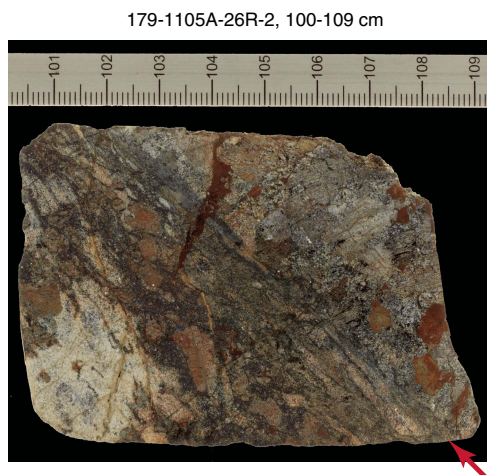
Figure F24. Example of a sharp structural contact (arrow) between a largely undeformed olivine gabbro and a crystal-plastically deformed olivine-bearing oxide gabbro (26R-2, 100–109 cm).
